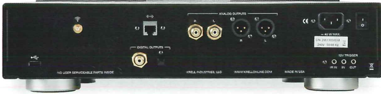
ABOVE: Single-ended and balanced (XLR) analogue outputs are provided, along with RCA and Toslink digital outputs. USB socket allows direct playback from a flash drive
