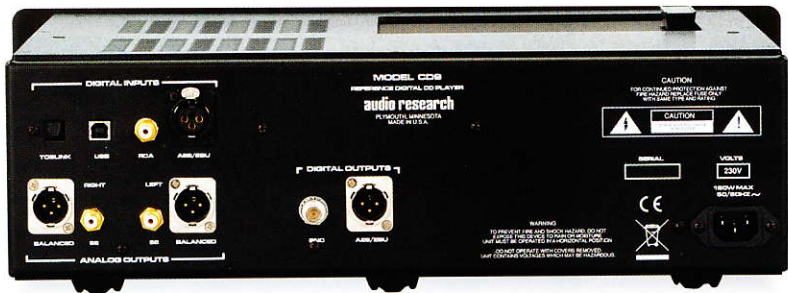
ABOVE: Balanced (XLR) and single-ended (RCA) analogue outputs are joined by USB, optical and coaxial S/PDIF and one AES/EBU digital input. Digital outs are offered too
