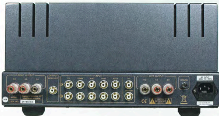
The DiaLogue Premium's rear panel features five line-level inputs as well as 8 Ohm and 4 Ohm 'speaker taps.
