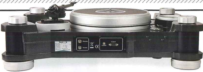
ABOVE: Pneumatic hoses from the outboard pump are connected to the air-bearing 'Flotation' and LP hold-down 'Vacuum' fittings while power and speed control are communicated via a multi-pin connector. Note the separate grounding post
