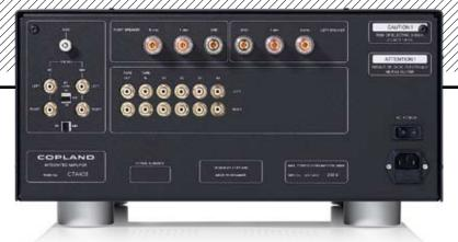
ABOVE: No digital inputs, but the CTA408 is equipped with a (solid-state) MM/MC phono stage and four single-ended line inputs feeding the (valve) pre/power stages. The 4mm loudspeaker outputs are notionally configured for 8 and 40hm loads
