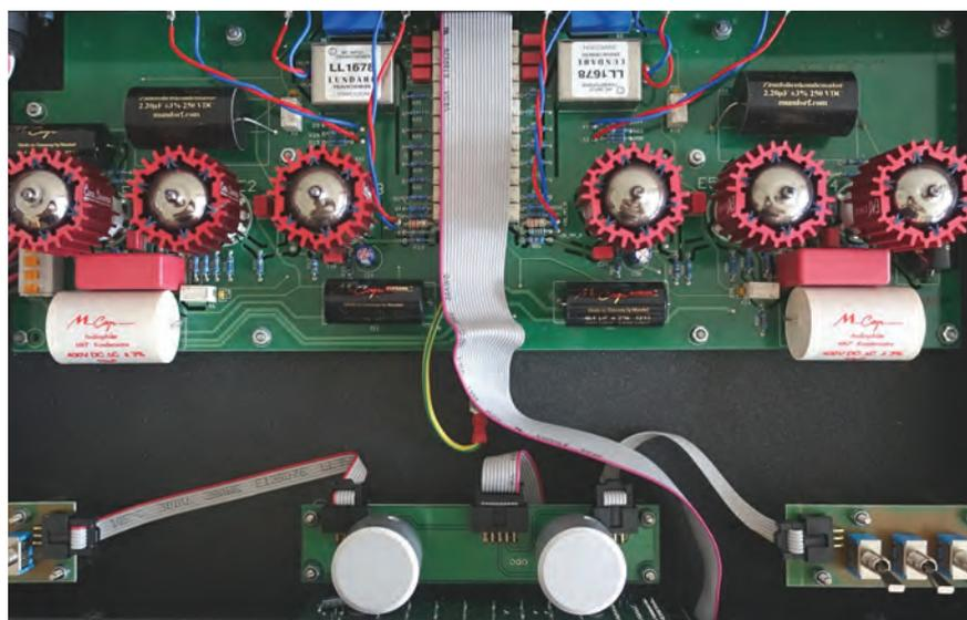
design, from the two-box configuration in aluminium alloy, to the low noise double-screened toroidal power transformer used in the supply. Following RFI filtering, the AC power is rectified to DC by fast-recovery, low-noise diodes that are fitted with noise damping resistors. Optimum isolation is assured using low feed-through FET regulation for the high voltage supply.
