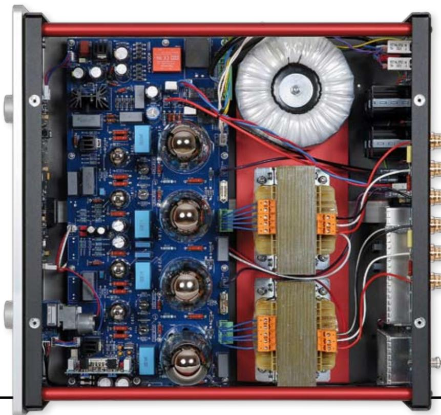
**RIGHT:** Linear PSU [top right] feeds a 12AY7 and 12BH7 triode per channel [left of blue caps] and pairs of KT150 output tubes [centre]. J-FET phono stage is separately screened [far right]; output transformers [right] have two secondaries
