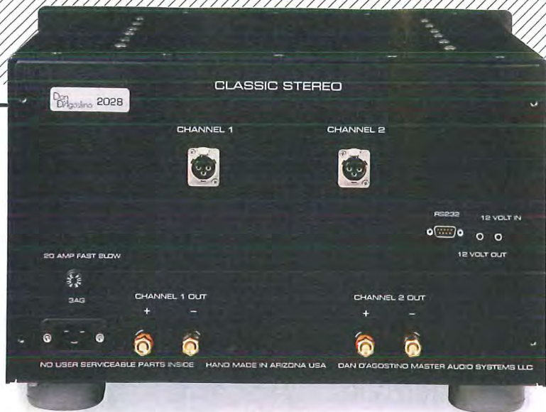
ABOVE: Balanced XLR inputs are joined by solid (not 4mm) screw-down speaker connections best suited for bare wire or spade adapters. Note 12V trigger comms
