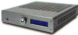
source friendly 110kohm, with 130pF of shunt capacitance. Channel balance at higher settings was accurate within 0.047dB at 20kHz, and generally about 0.08dB overall. The volume control has occasional missing codes where a 'click' does not result in a volume change, and where the resolution varies with level. At high settings you get 0.5dB steps; in the '30s' the steps are 0.8dB, with larger steps at very low volumes. This is not untypical of these ladder type controls.
