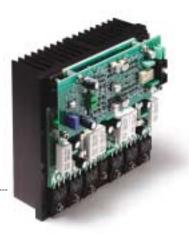
Easy Upgrades: Amplifier modules for the sixth and seventh channels can be added at any time.
