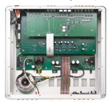
The Showcase processor employs fully discrete video circuitry. With bandwidth greater than 80 MHz, it ensures the integrity of all progressive and High Definition component signals, while still providing the convenience of on-screen display for all video signals.
