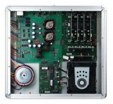
Two 24-bit ultra-high-resolution digital-toanalog converters per channel provide fully balanced operation with exceptional reproduction quality. The analog stage features Krell Current Mode,<sup>™</sup> discrete Class A, directcoupled, fully complementary circuitry.
