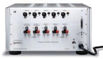
Both balanced and single-ended inputs are provided. 12VDC trigger input/output ports enable remote power on/off operation. A Multi Amplifier Throughput<sup>™</sup> (MAT) feature sends the signal to any or all channels from a single input connection for reduced wiring complexity in multi-amplified systems. A DB-25 input enables convenient single-cable connection of audio and control signals.
