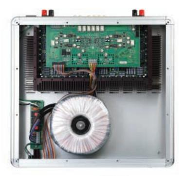
The power supply features a massive 800VA toroidal transformer. Extensive power supply filtering and decoupling between stages assure low noise and high stability.
