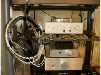
What turned out to be an unexpected practical advantage of the shelf-less approach was the ability to crisscross signal cables inside the structure through space usually blocked by solid shelving. This has merely the power cords 'exit' the back for altogether cleaner wire routing. The exposed cross brackets also lend themselves to things like Ikea kitchen hooks from which I hung headphones.
