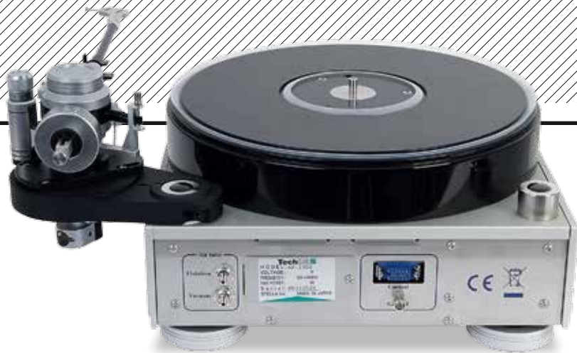
ABOVE: Pneumatic hoses from the outboard pump are connected to the air-bearing 'Flotation' and LP hold-down 'Vacuum' fittings while power, pump and speed controls are communicated via a multi-pin connector. Note separate ground post
