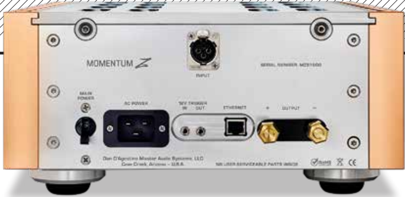
ABOVE: The wired Ethernet port allows access to service data – including operating voltages, temperature, bias, DC offset, 12V trigger status, and more – via a web browser. A balanced XLR in and solid metal binding posts (speaker cable/spades only) set the minimalist tone
