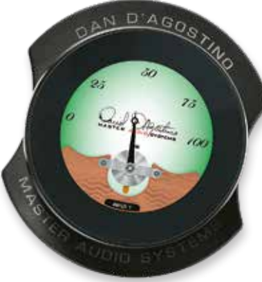
ABOVE: The C2Z’s alloy/Delrin (BT) remote, with LCD screen, offers control over most functions while mirroring the preamplifier’s front panel display
