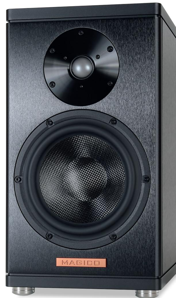
LEFT: The A1's sealed aluminium cabinet hosts a 28mm beryllium dome tweeter allied to a 165mm mid/bass unit. This composite carbon fibre cone includes a layer of 'XG Nanographene' to enhance its stiffness
