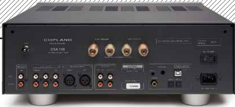
ABOVE: MM phono is joined by a tape loop, three line ins (two on RCAs, balanced on XLRs), a preamp out and single sets of 4mm speaker terminals. Digital inputs include coaxial, two optical and USB. Note hole for optional Wi-Fi/BT streaming adapter
