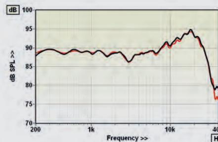
ABOVE: Forward response is flat through bass and mid, lifted through treble and drops steeply >20kHz
