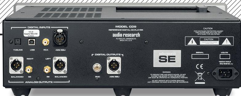
**ABOVE:** Balanced (XLR) and single-ended (RCA) analogue outputs are joined by USB, optical and coaxial S/PDIF and one AES/EBU digital input. These accommodate up to 192kHz/24-bit (no DSD, and optical to 96kHz). Digital outs are offered on BNC/XLR
