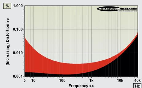
**ABOVE:** Distortion vs. frequency from 5Hz-40kHz re. 10W/8ohm (black, Direct; red, Balanced mode)
