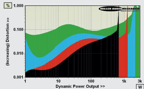
**ABOVE:** Dynamic power output versus distortion into 8ohm (black trace), 4ohm (red), 2ohm (blue) and 1ohm (green) speaker loads. Max. current is 53.4A
