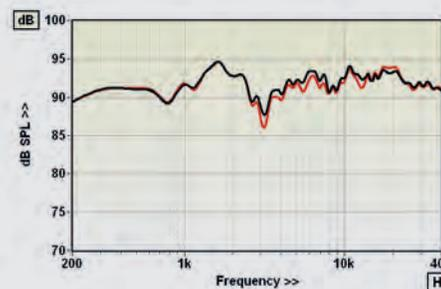
ABOVE: Pair matching is good while the peak at 1.6kHz and dip at 3kHz smooths out with distance
