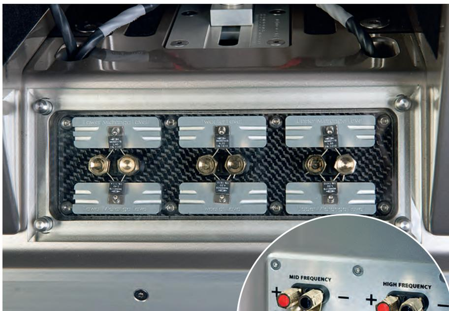
**ABOVE:** The resistor plate, which contains the protection and tuning resistors, is now located atop the bass cabinet for easy access. The high-pass mid/treble crossover is also mounted here
